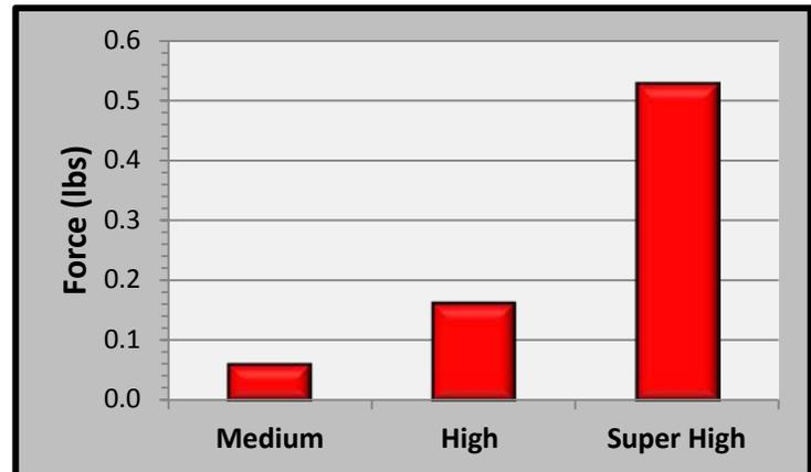
Loop Tack Testing of our medium, high and super high tack Adhesive Squares™ demonstrates **excellent adhesion** to stainless steel – increasing **product integrity** to give you **peace of mind.**
